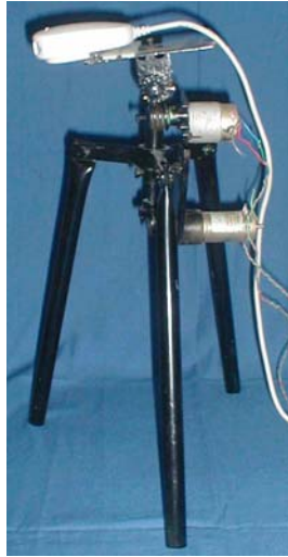
Figure 2. Pan-Tilt Camera Motor Configuration
