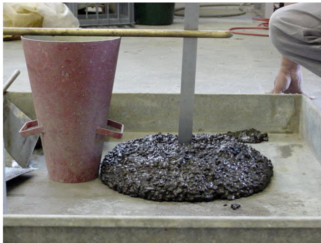
Figure 2: Workability of fresh geopolymer concrete (240 mm slump)
