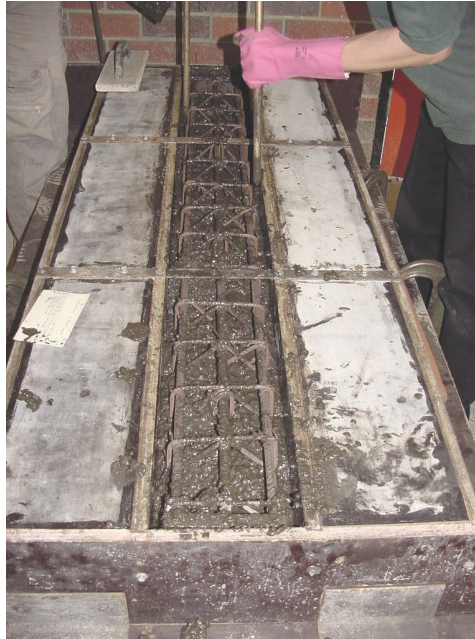
Figure 1: Manufacture of geopolymer reinforced concrete column
