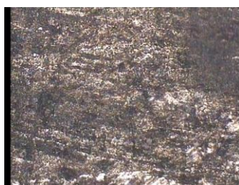
Gambar 11. AC-43100 (AlSi10Mg(b)) + 15% SiC* Sesudah di korosi larutan pH 7
