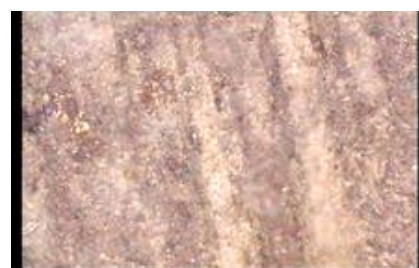
Gambar 7. Sampel 4: AC-43100 (AlSi10Mg(b)) + 15% SiC* Sesudah di korosi NaOH 0,1M
