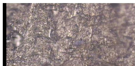
Gambar 15. AC-43100 (AlSi10Mg(b)) + 15% SiC* Sesudah di korosi kering suhu kamar (~ 270C)
