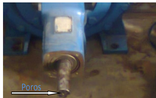
Gambar 3. Poros pompa
