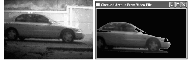
Figure 5. Example of Frame That is Failed to Pass The Segmentation Phase
