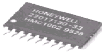
Gambar 1. Sensor magnet HMC 1002
