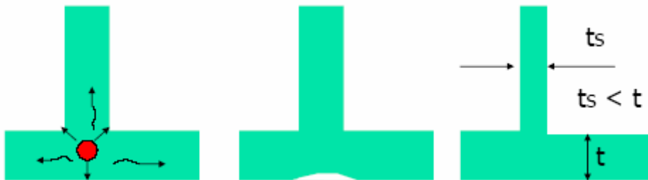
Gambar 2. Cacat Sink Mark
