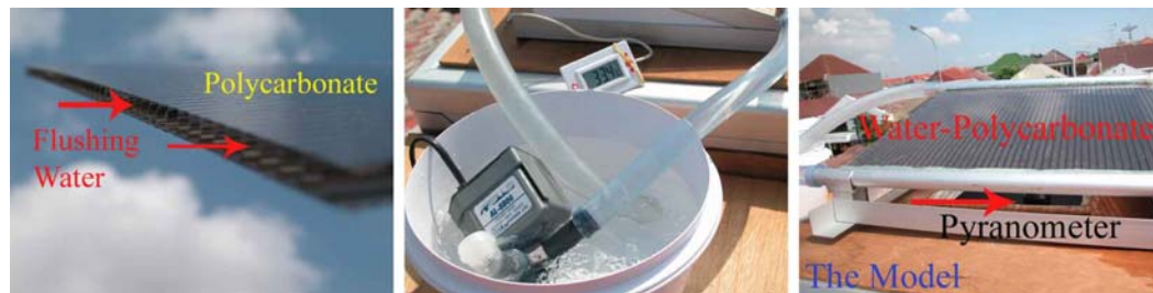
Fig. 5: The water-polycarbonate skylight device and measurement tools
